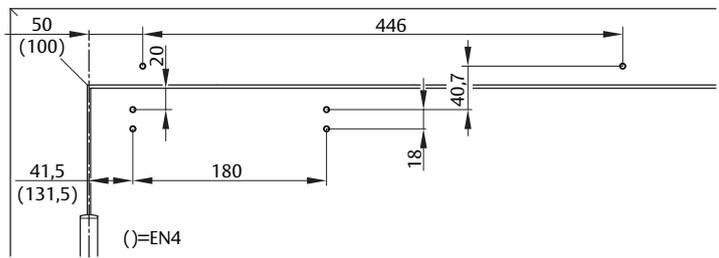
Installation dimensions with mounting plate for standard mounting on hinge side
