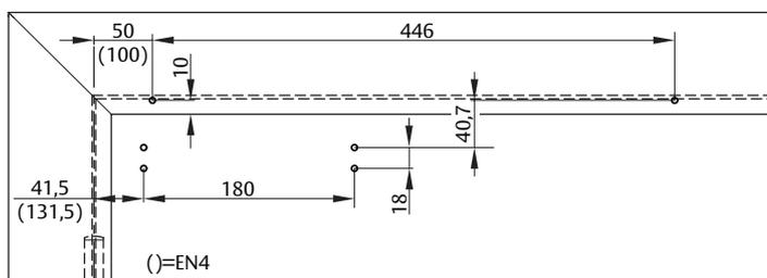
Installation dimensions with mounting plate for standard mounting non hinge side
