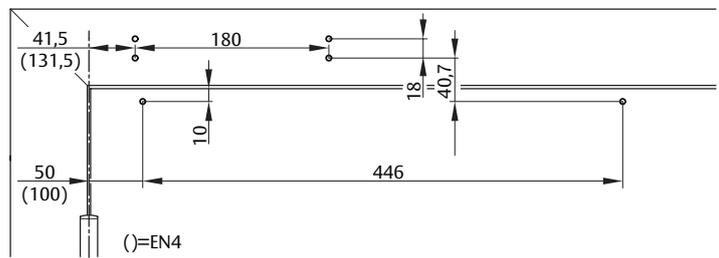
Installation dimensions with mounting plate for frame mounting on hinge side
