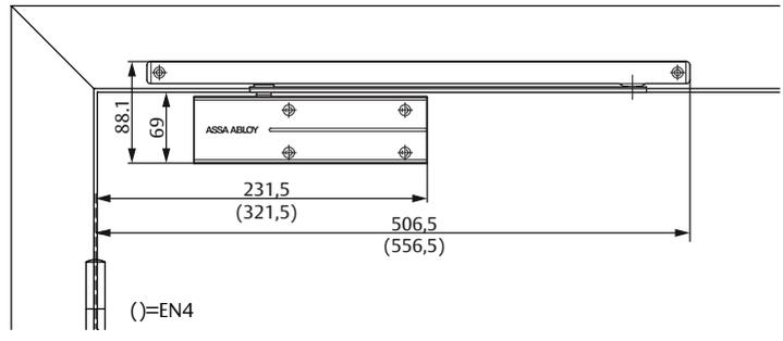
Space required on doors for standard installation on hinge side
