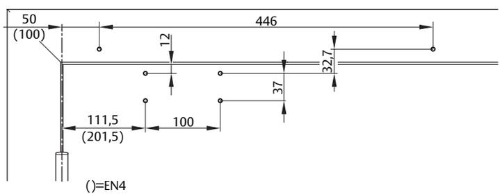
Installation dimensions for direct standard mounting on hinge side
