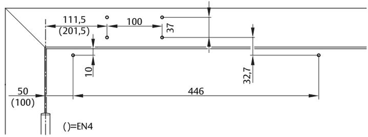
Installation dimensions for direct frame mounting on hinge side
