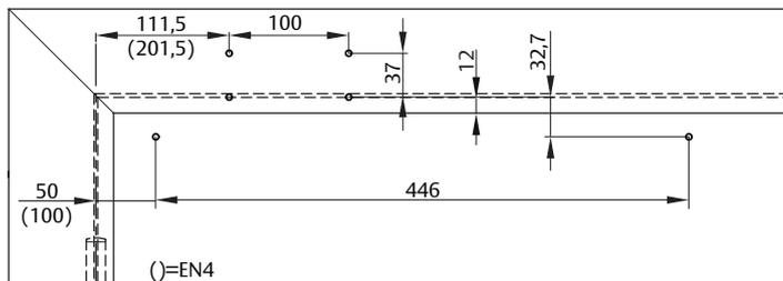
Installation dimensions when mounted directly onto the frame non-hinge side
