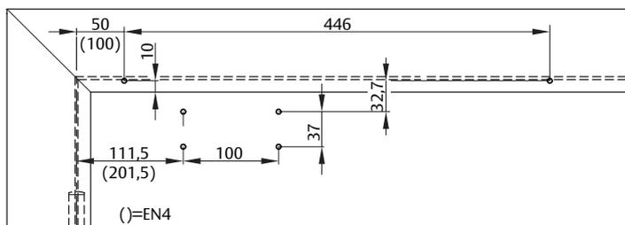
Installation dimensions for direct standard mounting non hinge side
