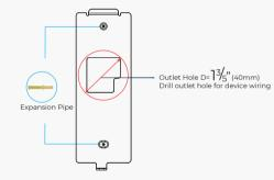
Please punch out the tail lines from the outlet hole before installing the mounting bracket and use the screws to fix the mounting bracket on the wall. Use the screwdriver to tighten thescrew follow the direction indicated, to complete the installation.
