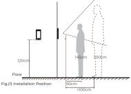
Suggested installation height (the distance between the lens and the ground) is 1.4m, as the recognizable body height range, 0.5m distance away from the device, is 1.3m-1.7m; the recognizable body height range, 1m distance away from the device, is 1m-2m. (There are some deviations)
