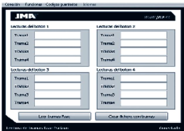
Press the 'Read FAAC screens' button to read the screens stored in the SR.
