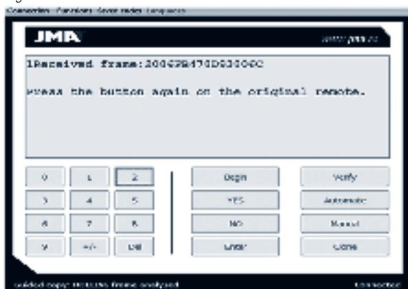
When the second screen requested has been sent, if the code has been decoded, it will display information about the type of remote, serial number, counter, personalisation and seed if these are required.
