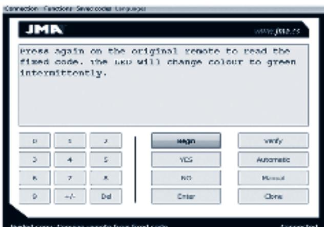
Once the code has been captured, press button 1 if the original remote is a 433 remote or button 2 if the original remote uses a variable frequency. In this second case, you must adjust the frequency once recording is finished.
