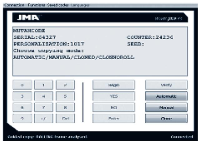
As when making a Guided duplicate, when the remote analysed is a fixed code remote it asks you to press 'Enter' to read the complete code from the start.
