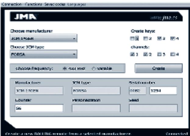
In the case of other manufacturers such as 1st GEN JCM, 2nd GEN JCM or GO, you need to select the type of JCM so that the second combination is suitable. The example shows the manufacturer '1st GEN JCM' type 'FORSA'. You can also see that 'Personalisation' and 'Seed' are disabled as this manufacturer doesn't use them.
