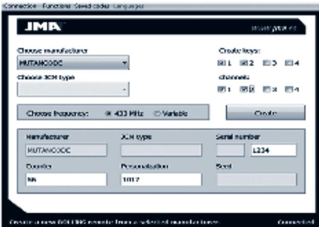
In the example displayed here, the manufacturer is 'Mutancode' and the serial and meter numbers have been entered. In addition, this particular manufacturer tends to have a personalisation number, so this value is entered if you know what it is. If no value is entered enter, zero will be allocated.
