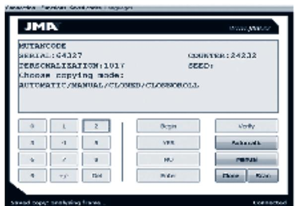
You can copy Automatically, Manually, or by Cloning and in some cases ClonNoRoll (Non-Rolling Clone) on rolling code remotes.
