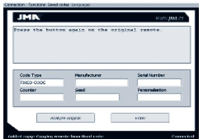
If you press the original again, the switch information is displayed (if it's a DIP-Switch remote,) along with the screen read.
