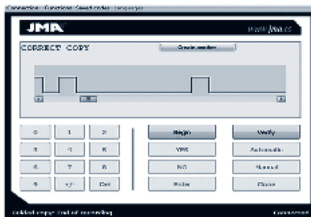
On pressing the 'Verify' button, a second window opens. It only displays the code that has been read while the remote recovers the code saved
