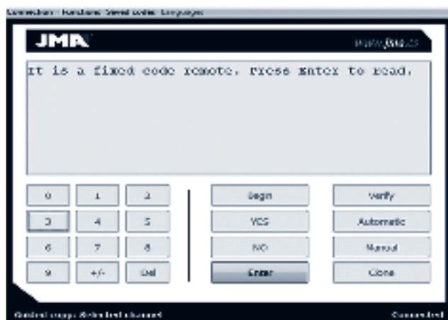
The remote will detect that it is fixed code and will ask you to press 'Enter' in order to read it. When you press 'Enter', the next screen opens, asking you to press the original remote so it can capture the code.
