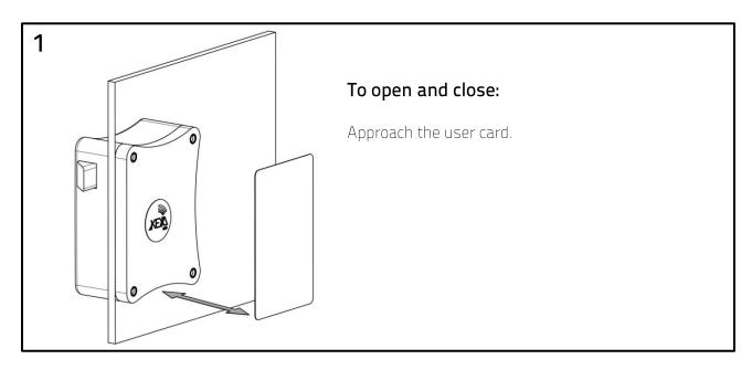
Access by transponder. The transponder code is erased every time the lock is opened, being available for a new user.
