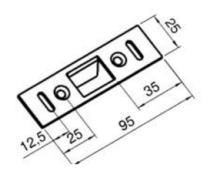
Sliding plate for operating the latchbolt with bent edge in the doors opening direction.
