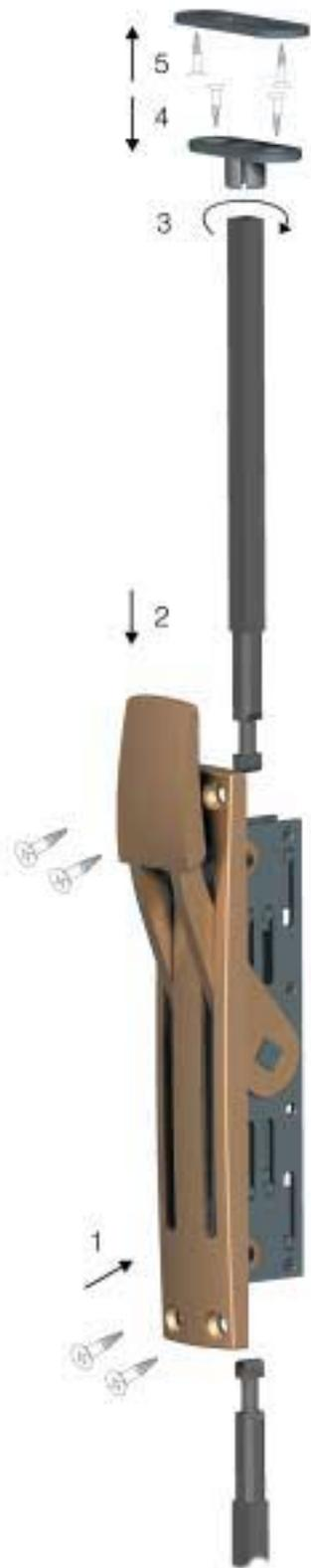
*Quick-bolt 3000 fitting diagram.*
