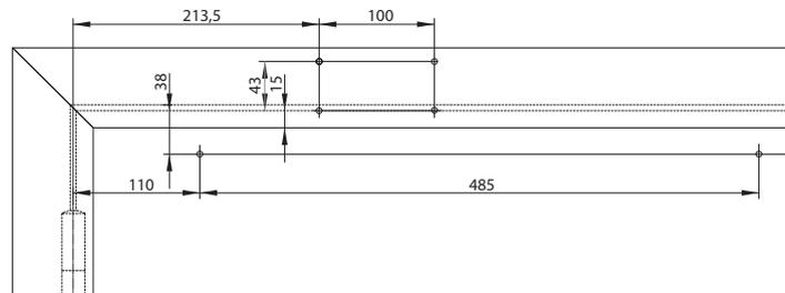
4 - Mounting on frame hinge side
