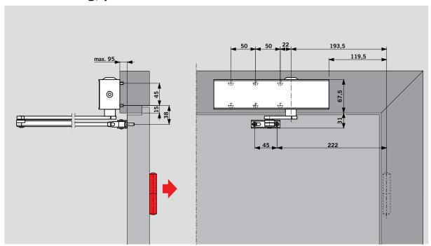
Door closers may only be fitted on the frame of fire doors if proved suitable for the individual door by the issue of an approval certificate from a recognised testing institution.
