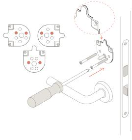
Step 4 - Use screws from step 2 to loosely attach the door plate. Use holes shown above depending on the chosen mounting angle. The rubber side of the plate faces the door. If a different length screw is required, cut the longer screws supplied to the correct length.
