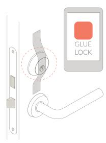
Step 1 - Download the **GLUE LOCK** App. Secure the lock cylinder on the outside of the door with sticky tape. This makes it easier whilst you fit your Glue Smart Lock.
