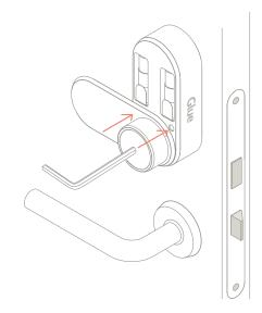
Step 8 - Holding the Glue Smart Lock against the door, screw the two screws behind the battery cover to the door plate. Use the thumb turn on the Glue Smart Lock to check the latch opens and closes smoothly, if not, return to Step 4.
