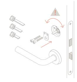
Step 3b - Replace with one of the three tail pieces supplied, that fits between the MIN and MAX lines. DO NOT ROTATE THE LOCK OR TAIL PIECE WHEN FITTING.
