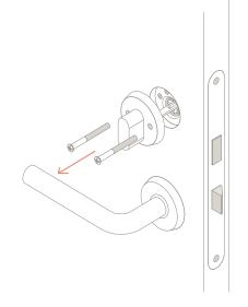
Step 2 - Remove the existing inside thumb turn by unscrewing the two screws in the thumb turn plate. Keep these screws as you will use them later, if they are long enough.
