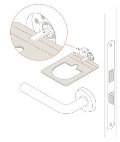
Step 3 - Measure the existing tail piece in your lock with the install template. The end should sit between the MAX and MIN lines. If it is the correct length, skip to Step 4.
