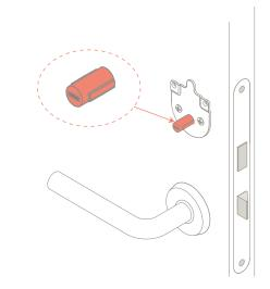
Step 6 - Slide the insert supplied over the tail piece.
