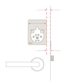
Step 5 - Ensure the door plate is straight by using the Glue Installation Template as a guide with the side of the door. Now fully tighten the screws, but do not over tighten. It is not a problem if the door plate does not fully cover the hole in the door.
