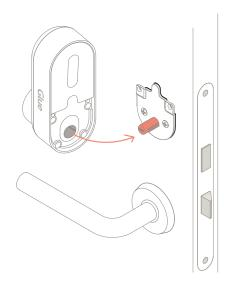
Step 7 - Turn the thumb turn on the Glue Smart Lock to the approximate centre, until the slots inside the turning section align with the ribs on the insert. Then slide the Glue Smart Lock over the insert onto the door plate.
