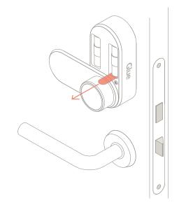
Step 9 - Check the lock is securely fastened to the door. If not, check all screws are tightened. Then remove the battery tabs. The light behind the thumb turn will flash twice.
