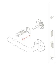
Step 3a - If the tail piece is too short, or too long, unscrew the D-plate and carefully remove it. Be careful not to drop the screws inside the door body.
