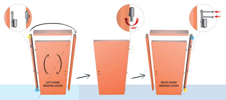
In the manufacturer's premises the male part of the hinge is fastened to the door panel, while the frame is pre-drilled. The female part can be affixed once the hand of the door is decided. In the building site, it just takes the rotation of the hinge body of 180° in order to change the hand of the door. Fixing of the frame part of the hinge by means of two screws and two pins, guaranteeing a perfect and long lasting loading capacity.
