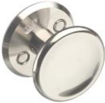
A classic door knob. Assa 496 is fixed and have no turn function. Used only as a pull handle. Made of brass with a diameter of the rose of  $\varnothing 52$  mm and  $\varnothing 50$  mm for the knob. Available in finish bright nickel, bright chrome, satin chrome, polished brass, satin brass, brown oxidised.
