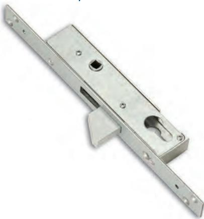
*Lateral lock with bolt and gear mechanism driven by handle square 8 mm. Lock of the handle by European cylinder key with 1 turn. One right/left hand. Galvanized finishing.*
