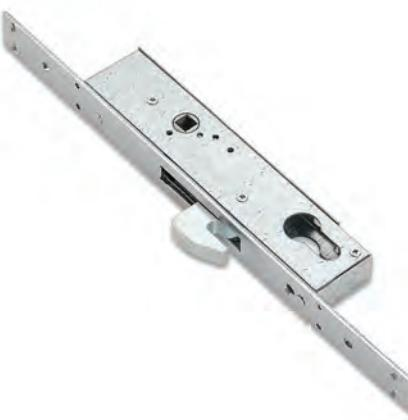
*Lateral lock with hook-bolt and gear mechanism driven by handle square 8 mm. Lock of the handle by European cylinder key with 1 turn. One right/left hand. Galvanized finishing.*
