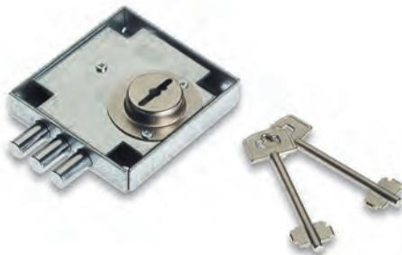
Lateral double ward lock 6 levers for little safe. Chromium-plated steel bolt with three pistons Ø 10 mm.
