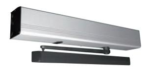
**ABLOY**<sup>®</sup> EMSW swing door operator works electro-hydraulically. It opens by motor and closes by spring. It is suited for external, internal, fire and exit doors, also for large and heavy doors.
